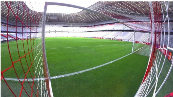
Pre corrected live feed showing classic lens distortion & curvilinear perspective artefacts
